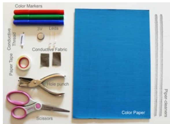
Figure 1. This educational soft circuit kit consists of: One color paper, Two Leds, Two piper-cleaners, Conductive thread, 3V batteries, Color markers, Paper tape, 2 pieces of conductive fabric. Tools are scissors and hole punch.
